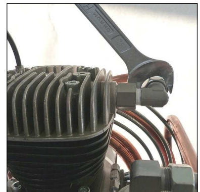
Fig. 6 - Connect pipe connections and tighten
