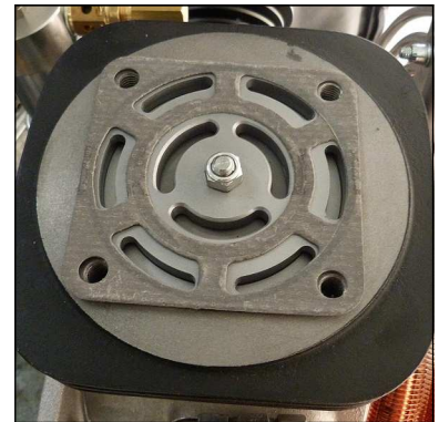
Fig. 4 - Place and align upper valve gasket
