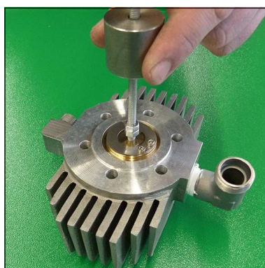
Fig. 4 - Remove inlet and outlet valve
