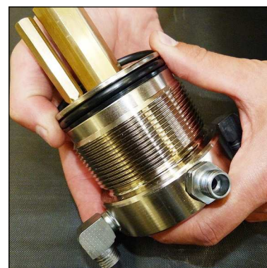
Fig. 4 - Change o-ring and back-up rings
