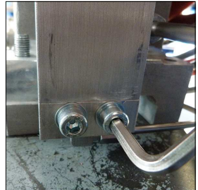
Fig. 1 - Loosen mounting screws
