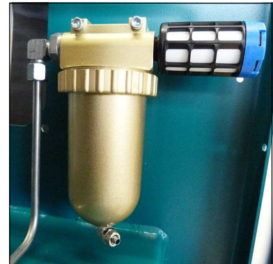
Oil / water separators final stage
