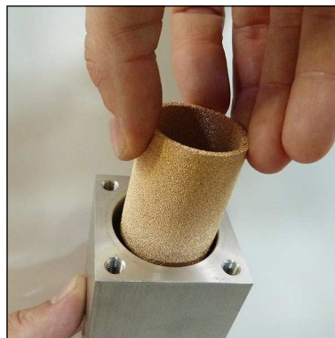
Fig. 4 - Change sinter filter
