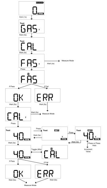
Fig. 7 Calibration - Toxic gases
