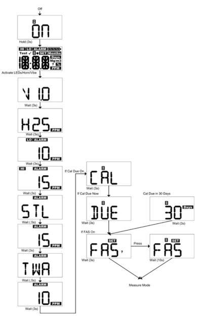
Fig. 4 Turning ON the instrument
