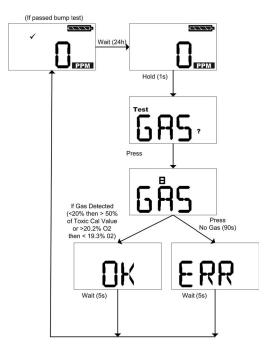
Fig. 6 Conducting the bump-test
