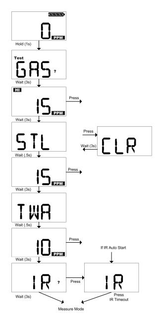
Fig. 5 Displaying instrument data (does not apply to the Steel Mill Version)
