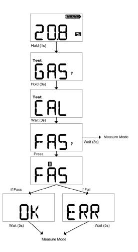
Fig. 8 Calibration – Oxygen
