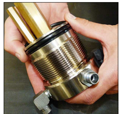
Fig. 4 - Change o-ring and back-up rings
